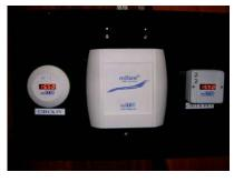
Working hours recording terminal device (ITGsr-05 with ITGant-7 readers) provides accurate records of employees arrivals and departures from the company. Abuse by the employees can be reduced to the minimum by placing the network video camera to survey the spot arround the RFID readers. Video camera provides snap-shot of employees checking in or out.
