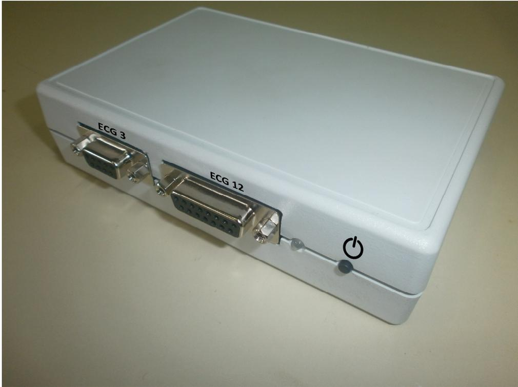
Fig. 1. Front side view of the *ECG 1410* Calibration Unit.
