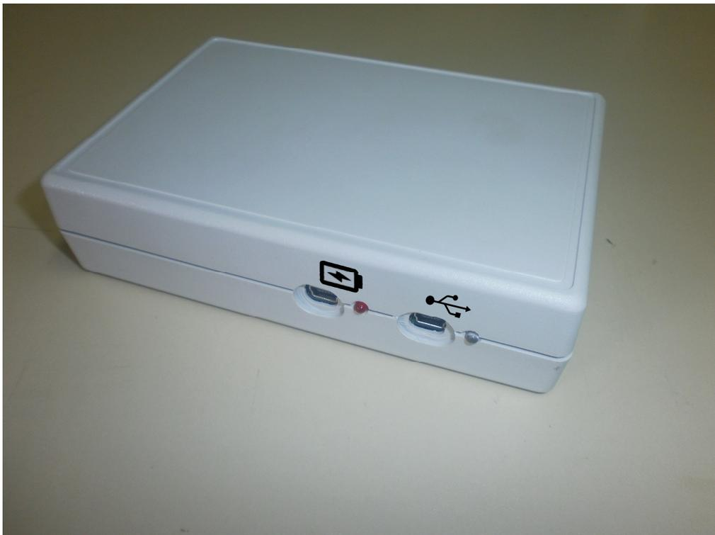
Fig. 2. Rear side view of the *ECG1410* Calibration Unit.
